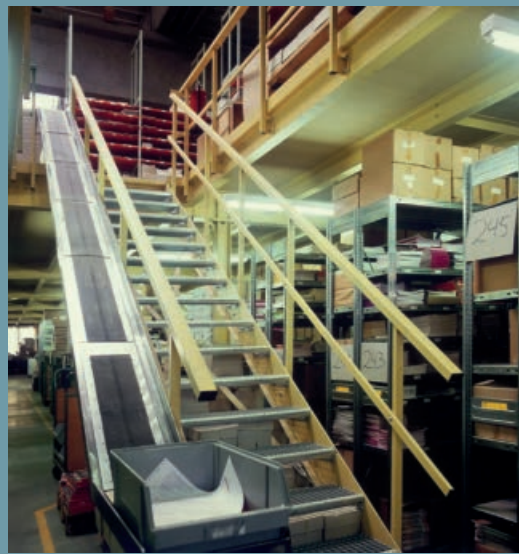
Solid storage platform with outside staircase and conveyor systems for boxes. High spans allow much freedom of movement under the platform.
