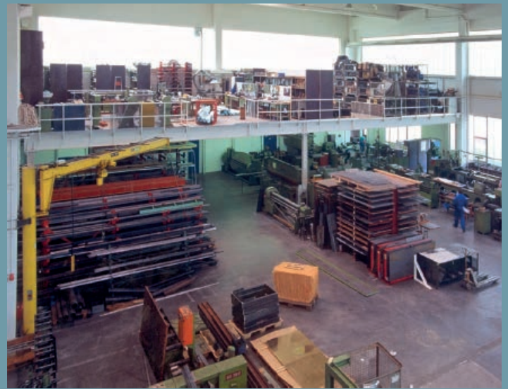
Doubling the area in the steel industry. Top and Bottom work-spaces. Load of 1,000 kg/sq. m.
