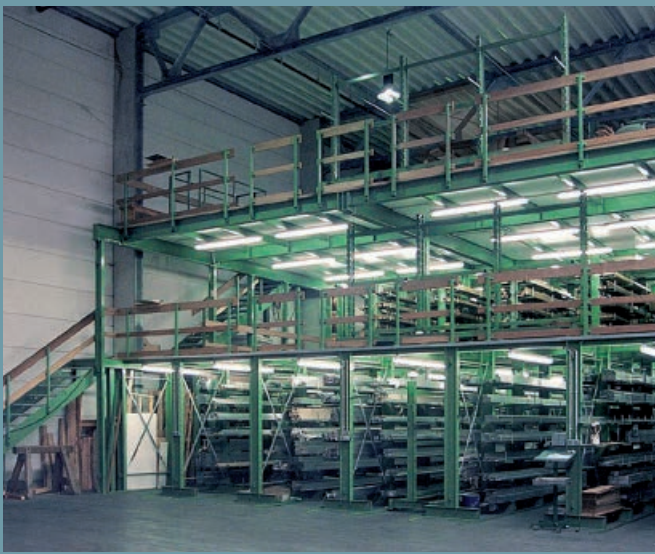
Cantilever arm storage platform in metal warehouse. Storage of profiles in cantilever racks over 2 floors. Top level for packaged goods and solid piled storage.
