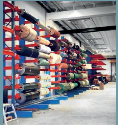
Cantilever racking with special fittings for the storage of rolls.
