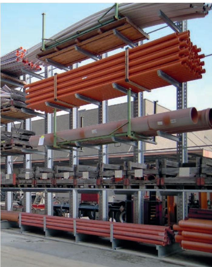
Plastic piping in the cantilever rack as an outdoor warehouse – floor and first storage level as a manual commissioning area, partially fitted with metal decking for special pallets.
