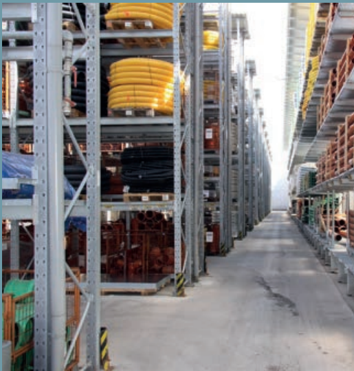
Pallet racking for the storage of plastic tubes and piping
