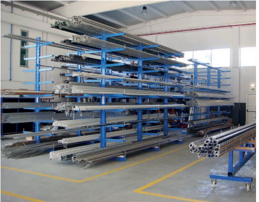
Manually operable cantilever racking for the storage of aluminium and plastic in a window manufacturing plant
