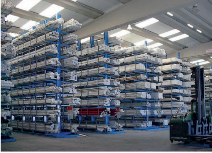
Narrow aisle system for the storage of stillages – servicing with a multi-directional lift truck.
