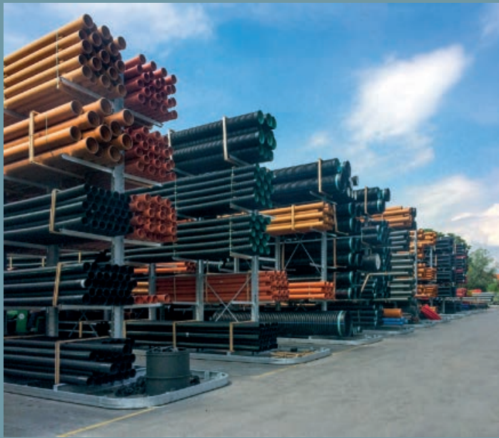
Outdoor storage of plastic pipes in the wholesale trade. Galvanized cantilever racking with guide rails for multi-directional lift truck.
