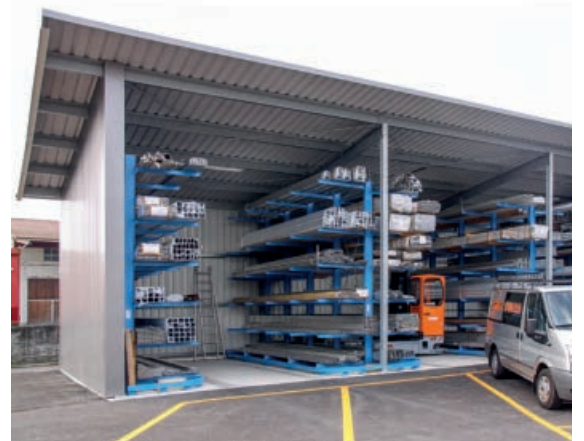
Cantilever racking in an open warehouse – serviced with a multi direction forklift
