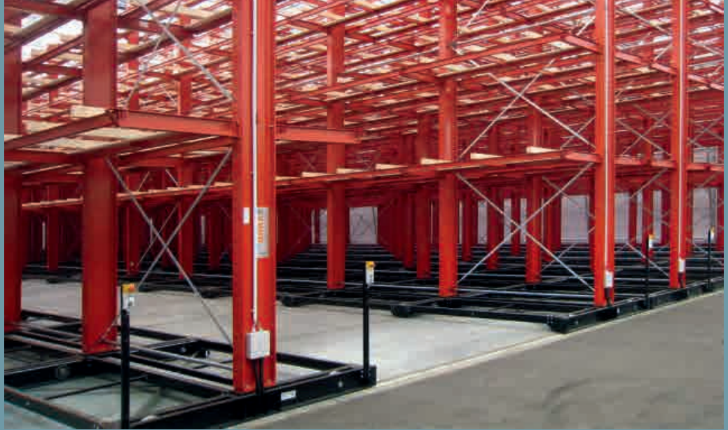
Mobile rack system unladen. Electrically operated by pressing a button for each individual traversing carriage
