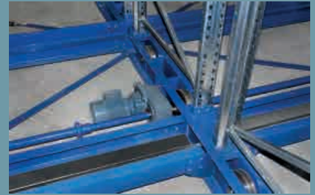
Traversing carriage with electric motor and drive wheel.
