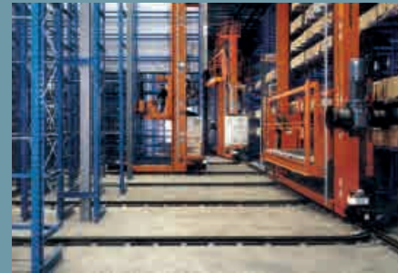
Rail mounted rack riser trucks during a change of aisles
